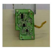
The iR1200 series is also fitted with a serial number PCB that is located on the side frame of the machine at the rear.
