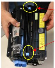
Once the tool has been fitted the drum can then be separated from the developer assembly. The two tabs highlighted in the diagram need to be released so that they are in the position shown below.
