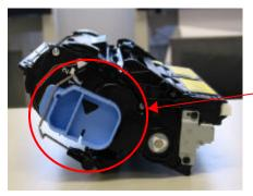
Before removing the drum assembly. away from the dev. assembly. It is important that the drum tool is fitted as shown. This locks back the shutter away from the OPC surface of the drum to prevent any damage to its surface.
