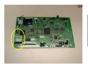
In addition to the serial number PCB the machine is also fitted with a counter memory PCB mounted onto the IP. If the IP is replaced be sure to swap the memory counter over to the new IP
